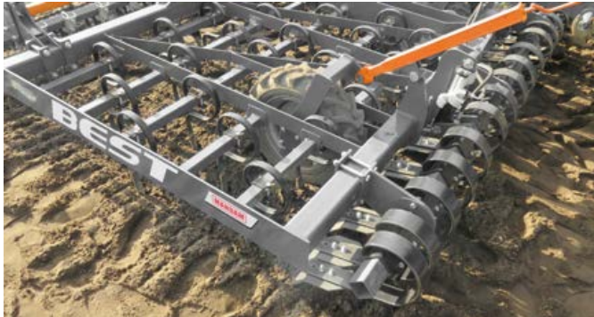
STRAIGHT TINE 32X12 MM (STANDARD)
